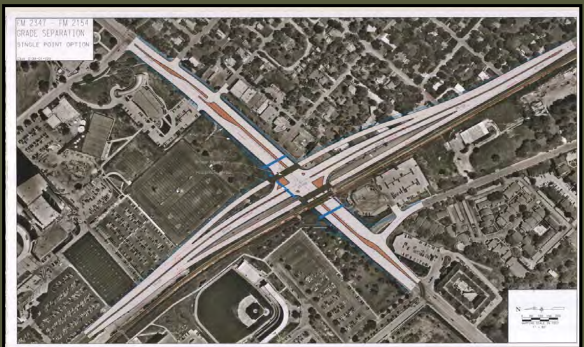
Figure D.1: Proposed grade-separated intersection. Source: TxDOT.
