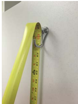
RR Violation 5 - The hooks in the accessible toilet compartments in the Southwood Community Center are too high at 64".
