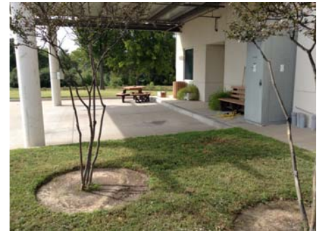
AR Violation 4 - No accessible connecting route is provided to serve the picnic table provided at the covered service entrance on the south side of the building.
